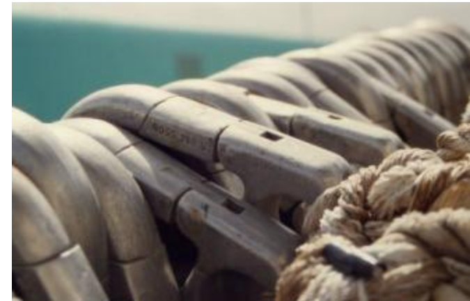
Stainless steel roller snap rings (Figure 5 in Itano 2003)
