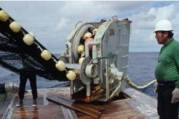
Retractable deck mounted power block (Figure 19 in Itano 2003)
