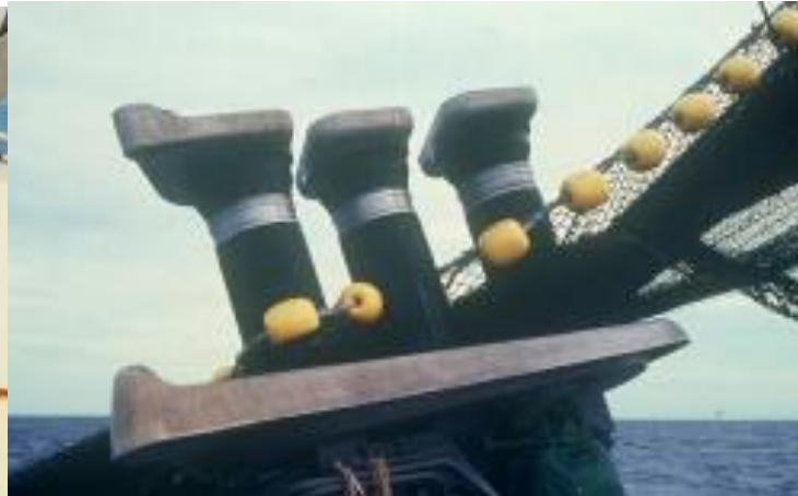
Triplex power block (Gillett) (Figure 14 in Itano 2003)
